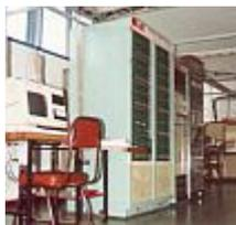
The META II spectrum analyzer at the Instituto Argentino de Radioastronomía control room. The new data acquisition system allows to expand the instantaneous bandwidth from the original 400 kHz to 2 MHz and to make integration of the frequency windows over several hours. The maximum spectral resolution is of 0.05 Hz and the available observing frequencies are 1.4; 1.6 and 3.3 GHz.
