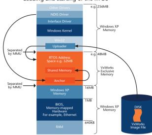
KUKA Controls' VxWin utilizes the x86 MMU to protect VxWorks memory from Windows XP.
