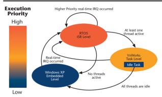
KUKA Controls' VxWin assures complete execution of all real-time tasks before switching back to Windows XP.
