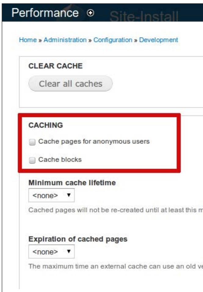
Figure 2. Configuration for Page and Block Cache
