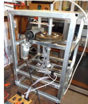
Fig. 3 Picture of the antenna rotor under development.
