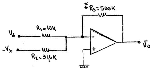
$$V_o = -\left(V_d \frac{R_3}{R_1} + V_x \frac{R_3}{R_2}\right) = -(50 V_d + 15,8 V_x)$$
