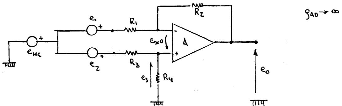
$$e_3 = (e_{1c} + e_2) \cdot \frac{R_4}{R_3 + R_4}$$
