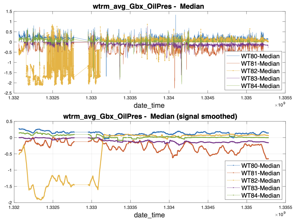
Figure 9. At the top, the residue of the signals wtrm_avg_Gbx_OilPres is depicted. The same signals smoothed by a 50-sample moving average filter are depicted at the bottom.
