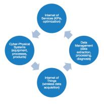
**Figure 1.** The structure for predictive maintenance in Industry 4.0.
