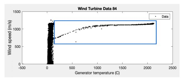
**Figure 2.** Erratic behaviour of the wind turbine 84 for the wind speed and the generator temperature variables.
