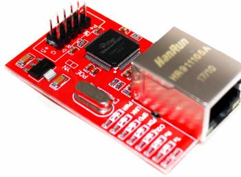
Figura 3.1: Chip Ethernet W5100
